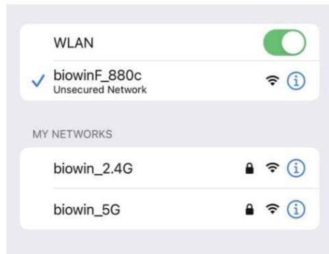
3. Open the mobile phone "Network Settings" to find the corresponding WiFi name, and click Connect; If the phone is connected to other WiFi, you can disconnect it first until you find the WiFi hotspot of the robot. The WiFi module starts for about 5s. **Note that if the pop-up window "The current WiFi is unavailable, do you want to continue using this WiFi?", you need to select "Use".**
