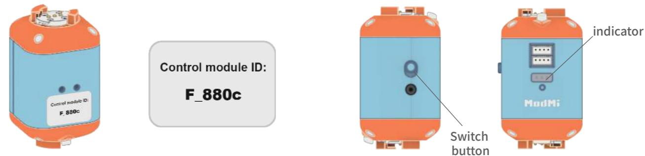
1. Find the robot id on the silver label paper of the F module. The id starts with "biowin", and the last bit is the corresponding control module type. For example, F module is "biowinF"+others.
